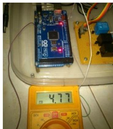
Image 4.2 Arduino Digital Output Pin Testing At HIGH Conditions
