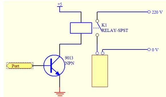
Image 3.4 Driver Circuit Water Machine and Electrical Valve
