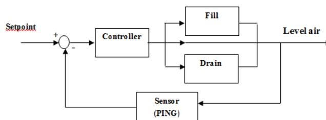
Image 3.1 Altitude Control System Block Diagram Water Pond
