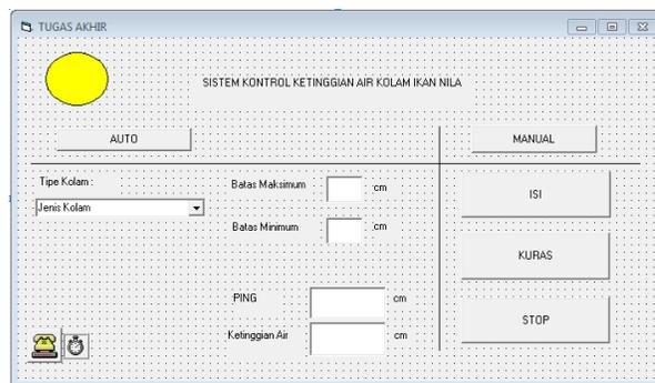
Image 3.7 Interface Control System Altitude Tilapia's Pond
