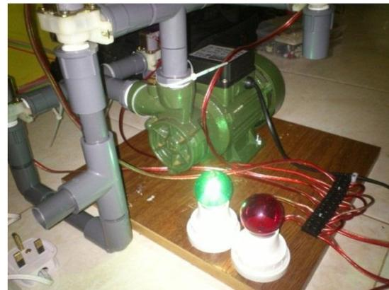
Image 4.9 Filling System Water Pool Is On When Press the ISI Button
