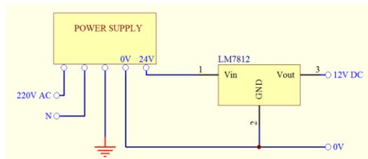
Image 3.3 Regulator 12V DC Circuit
