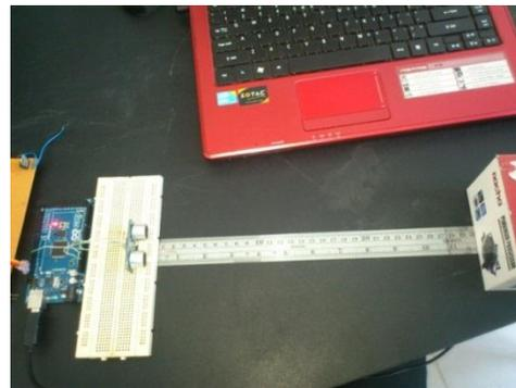
Image 4.6 Distance Measurement Using PING
