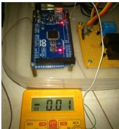
Image 4.1 Arduino Digital Output Pin Testing At LOW Conditions
