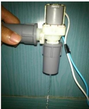
Image 4.5 Testing the Electric Valve
