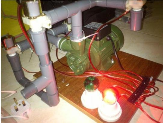
Image 4.10 Draining System Water Pool Is On When Press the KURAS Button
