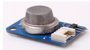
Gambar 5. Fisik Sensor MQ-2 (Moch. Rifai Syambara, dkk, 2014).
