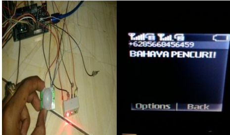
Gambar 19. Pengujian Sensor Passive Infra Red
